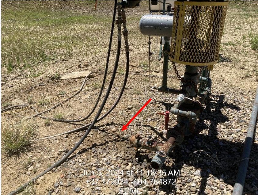
Photo 5 – Stained soils at wellhead
