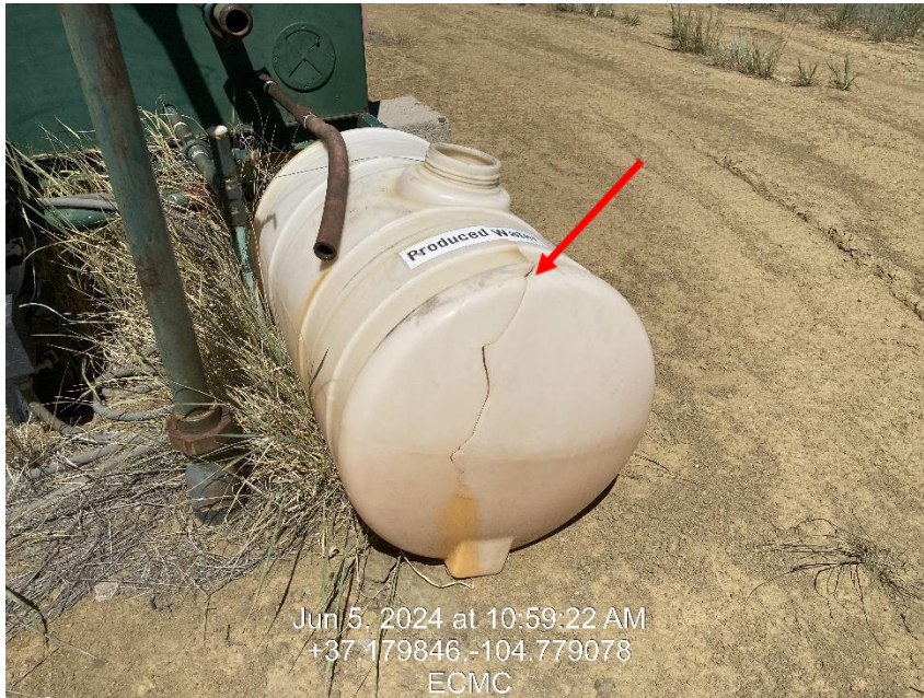
Photo 3 – Tank near Meter House broken
