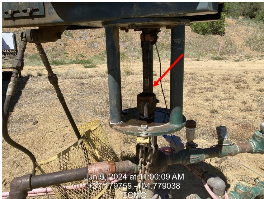
Photo 5 – Leaking packing
