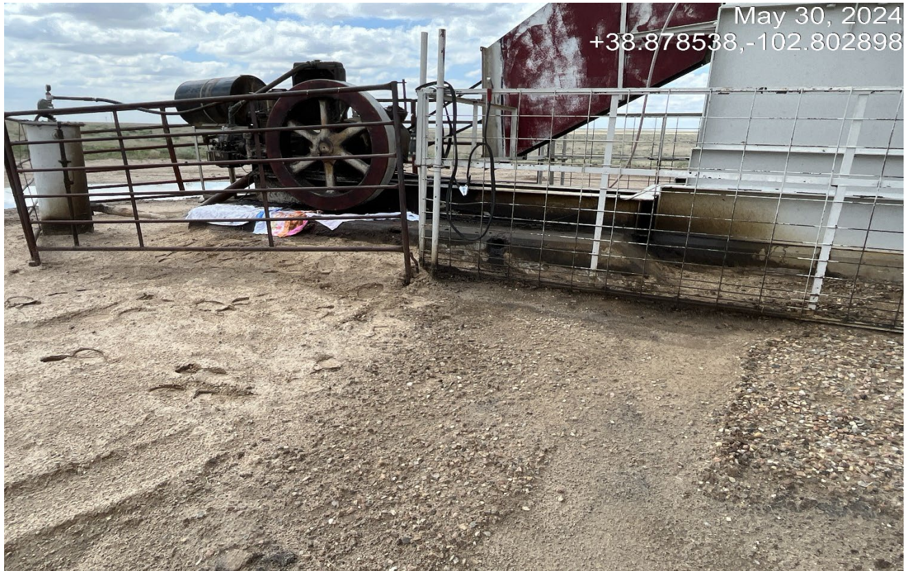
Photo 5. The pumpjack engine is still leaking oil and there
