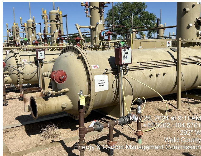
LO/TO Separator for Maintenance
