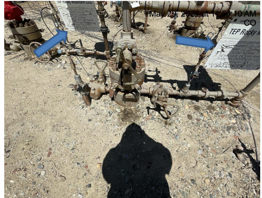
Photo # 8665 Multiple wellhead signs weathered/fading & cracking & starting to become illegible
