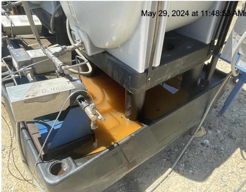
Photo # 8667 Failure to maintain chemical BMP/chemical containment full of fluid & not sufficient to contain possible spill
