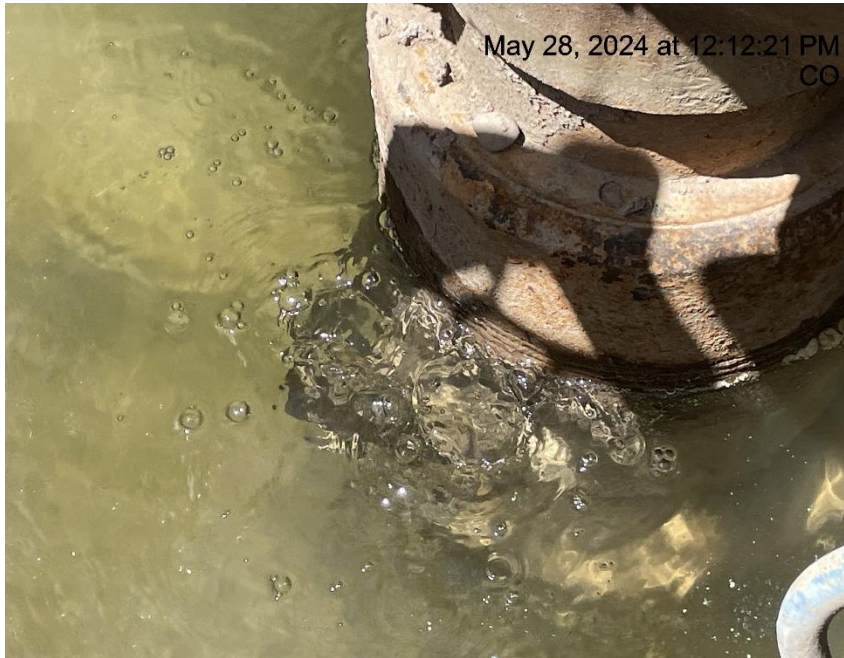
Photo # 8471 Possible wellhead leak/gas bubbling up around wellhead through water in cellar
