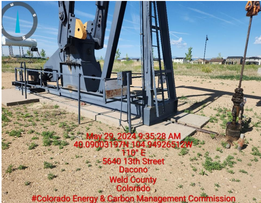
Photo 7 well head sign faded and blocked by electric panel
