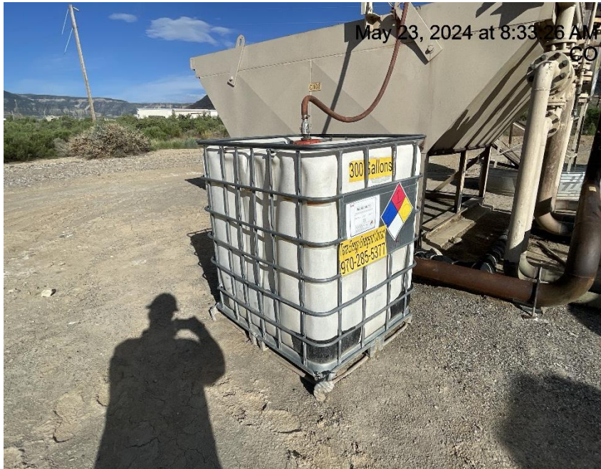
Photo # 8065 Chemical tote on location lacks BMP's/does not comply with CECMC Stormwater rules
