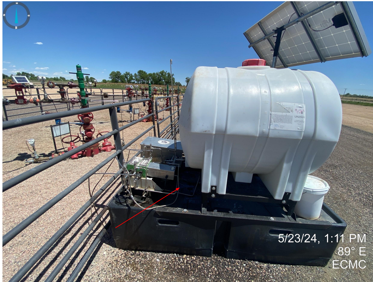
Photo 36. Free fluids observed within secondary containment need to be properly disposed of.
