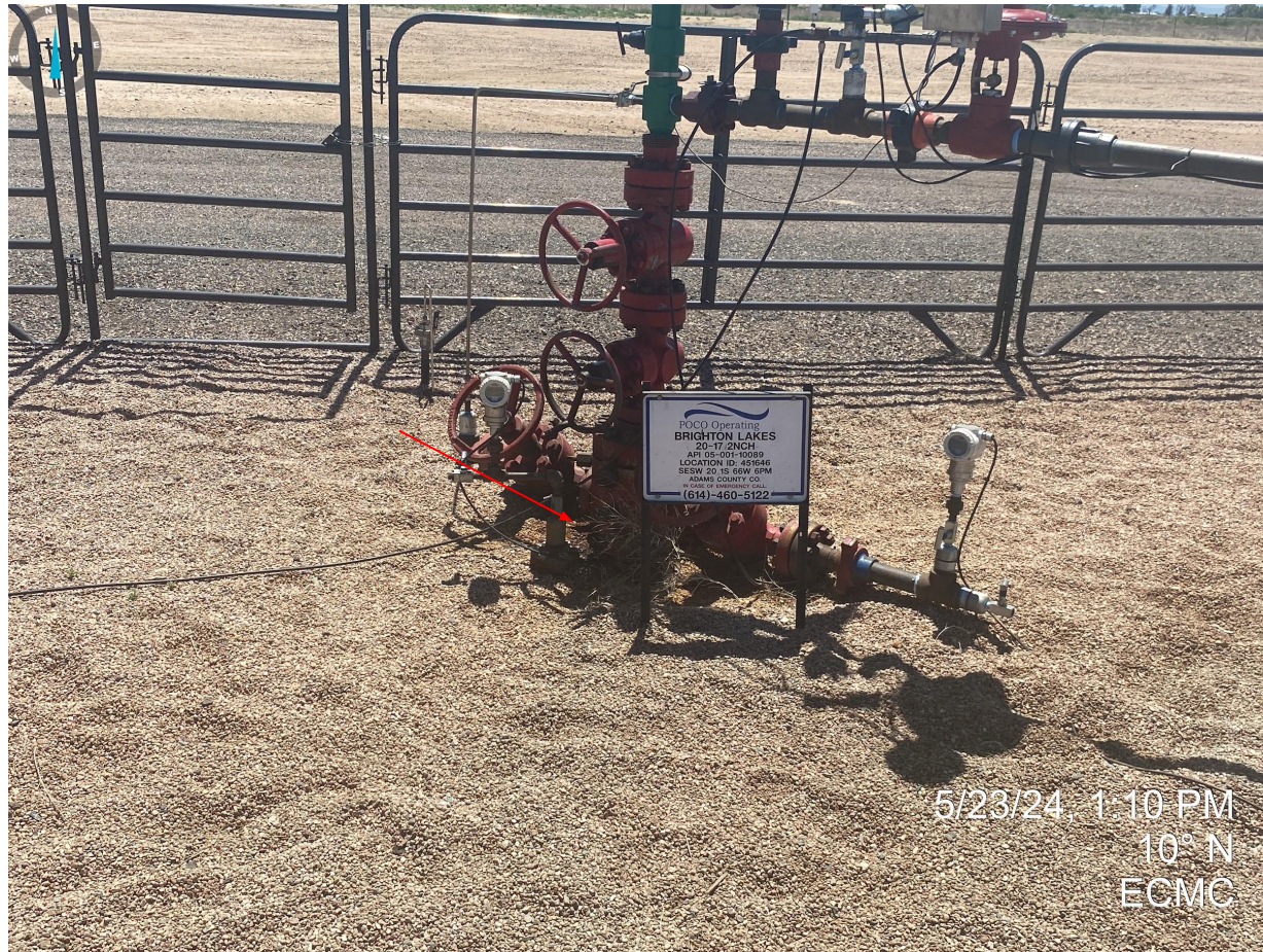
Photo 34. Stained soil observed near wellhead need to be properly disposed of per Rule 905.e.
