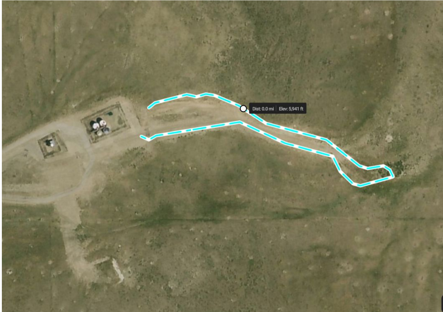
Photo 5. The photo was taken from onX imagery of the tank battery location. The photo illustrates the mapped boundary of erosion of the location. Sediment was observed approximately 550ft off location.
