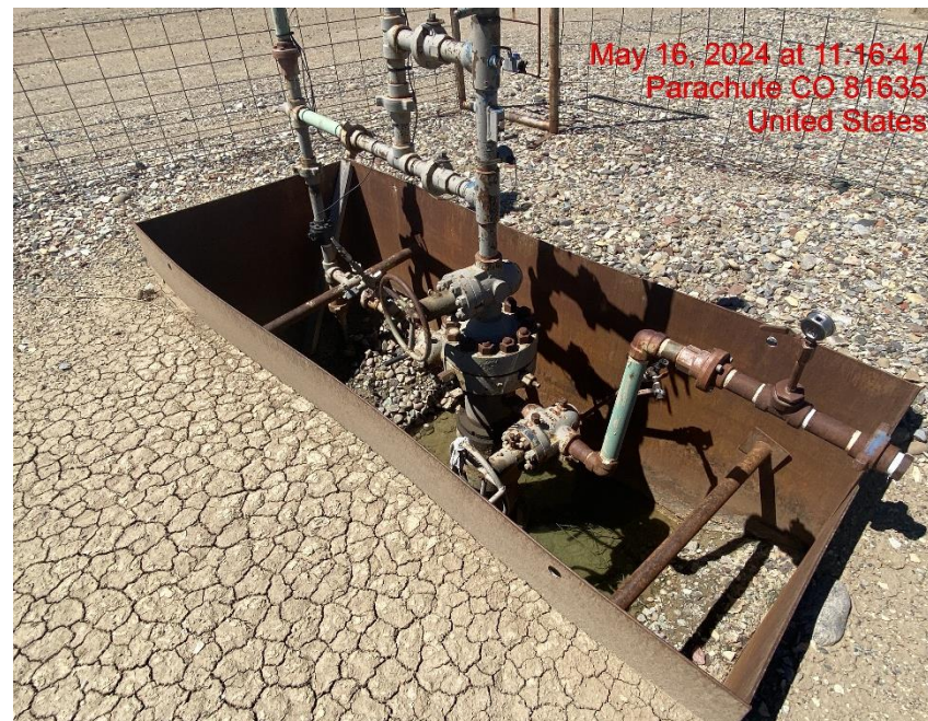
Uncovered Wellhead Cellar – Photo #01264
