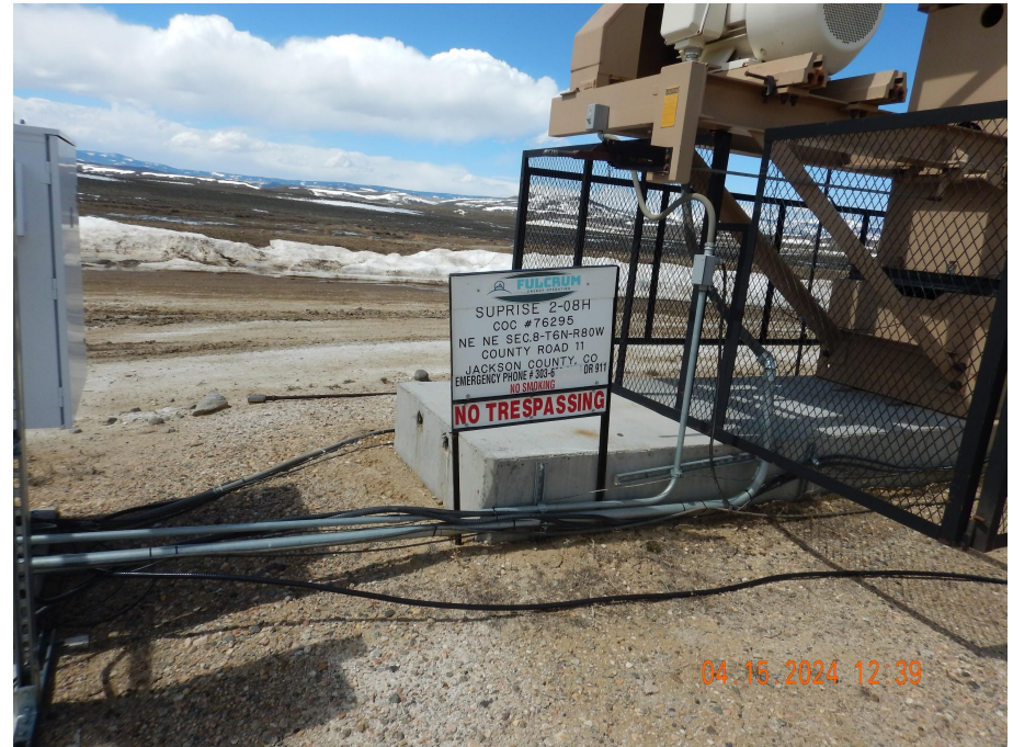
Photo 3. Photo taken from the wellhead, facing West. Photo illustrates the well signage that lacks API information.
