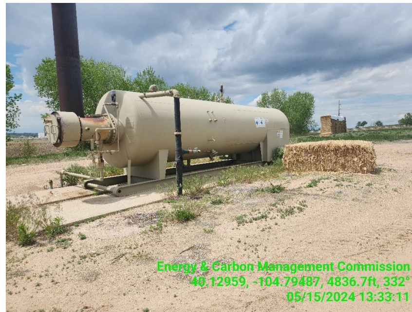
Photo 12 Vegetation around the Heater Treater need to be addressed.
