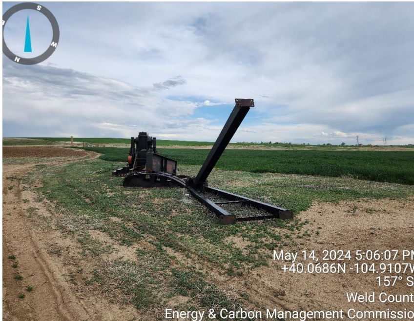
Photo 3 disassembled pumping unit
