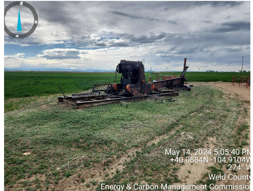
Photo 4 disassembled pumping unit
