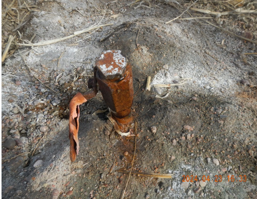
7. View of continued water seep at valve and plug.
