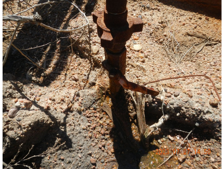
4. Closer view of hammer union and valve 7/27/2023 inspection.
