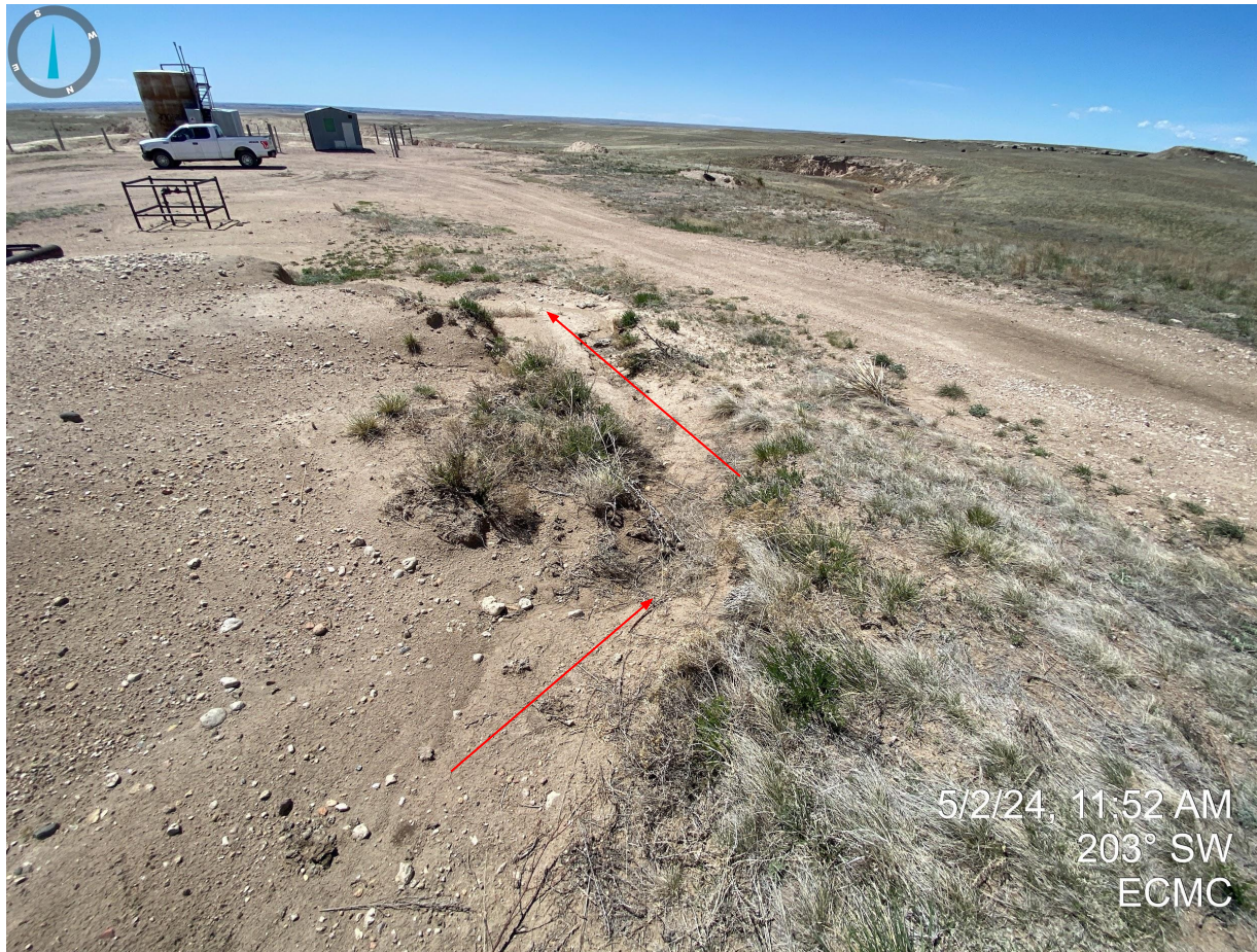
Photo 2. Areas experiencing erosion degradation throughout the production areas do not appear to have been repaired/stabilized and there is no evidence of stormwater controls measures/BMPs having been implemented.
