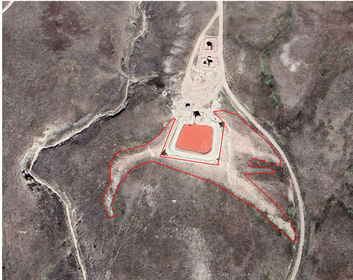
Photo 29. Google Earth aerial imagery taken circa 09/2023. Image illustrates the approximate extent of the impacted salt kill areas, highlighted in red. Note: the red outline is only an approximate extent as the Operator is required to fully delineate the extent of the salt kill impacts.
