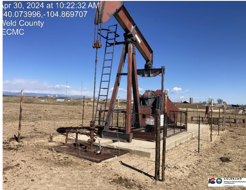
Pic 1 wellhead / pump jack
