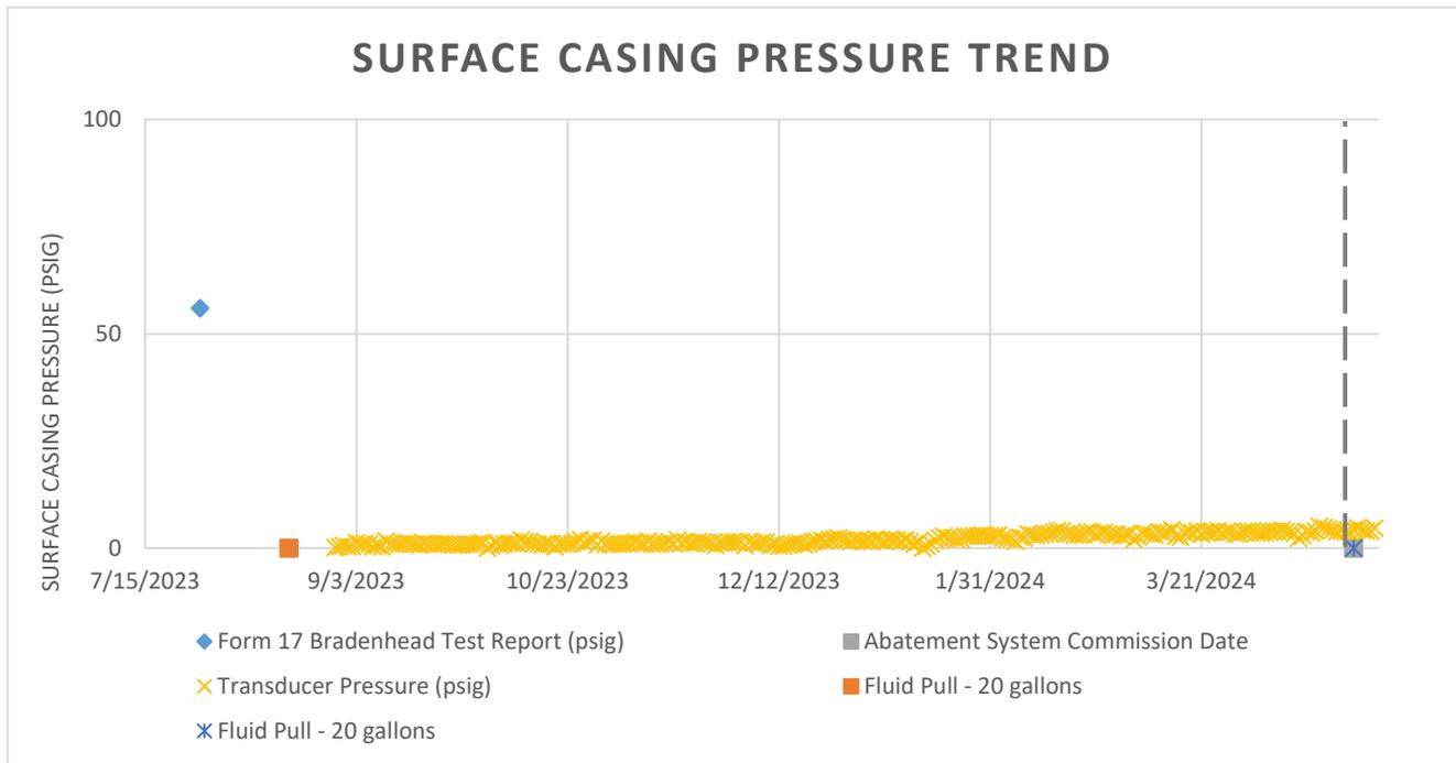
**Comments:** 2023 ad hoc test had 56 PSI gas flow that blew down to 0 psi after the first minute, water started after 3 minutes and trickled for remainder of test. Bradenhead gas determined to be thermogenic gas with somewhat similar composition as the production gas sample. PDC attempted fluid displacement to remediate bradenhead pressure but could not reach further than 10' with hose. PDC has opened this well to facility abatement.
