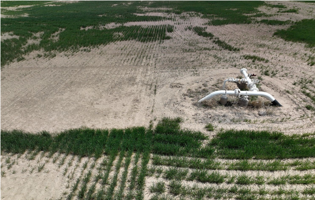
Photo 5. Facing east down toward the abandoned wellsite. It appears there is no crop growth coming up to the left of the pipe risers.
