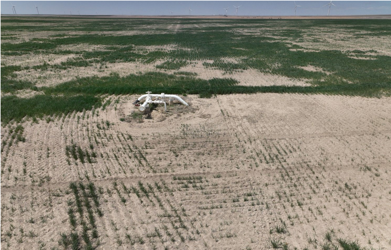
Photo 3. Facing west toward the abandoned wellsite location. There are pipe risers and lines that have not been abandoned and removed.
