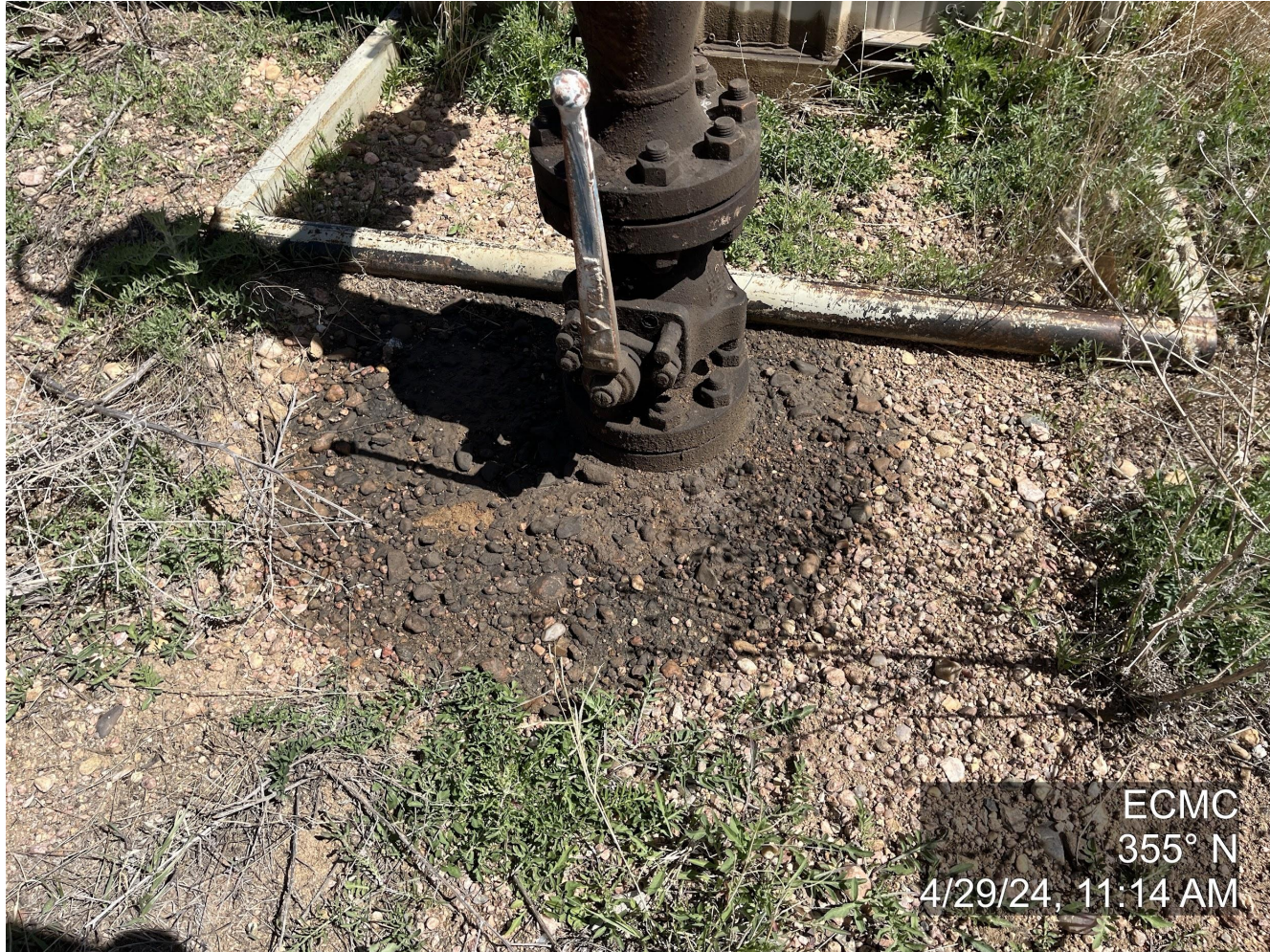
Photo 5. The photo was taken at the tank battery location facing North. The photo illustrates soil staining at the meter shed.
