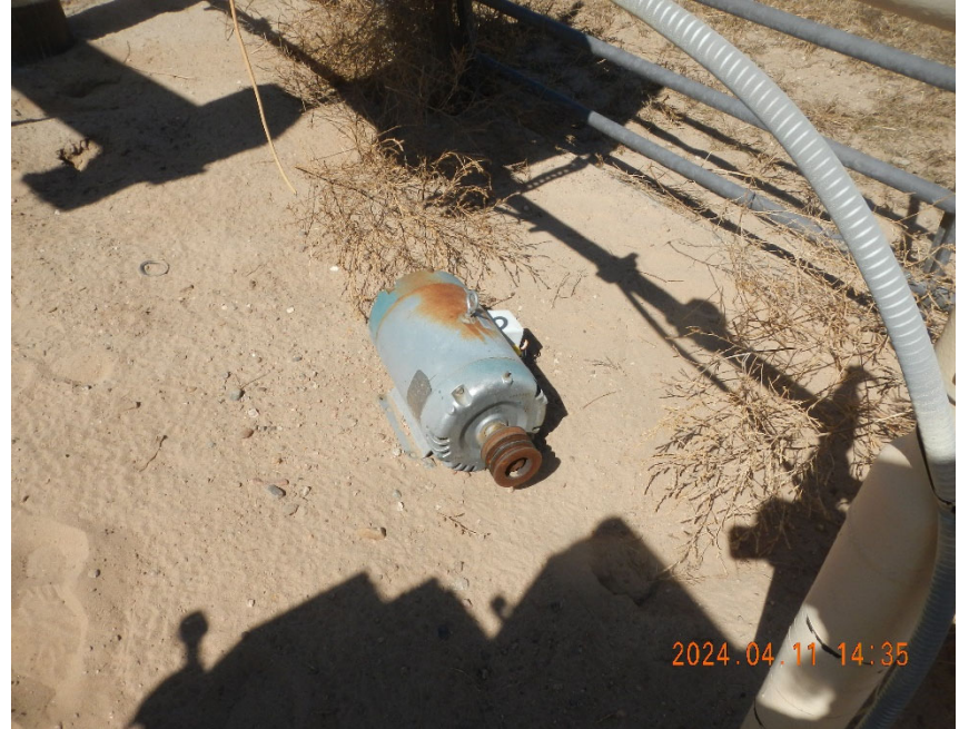
6. Electric motor on ground inside well fencing.
