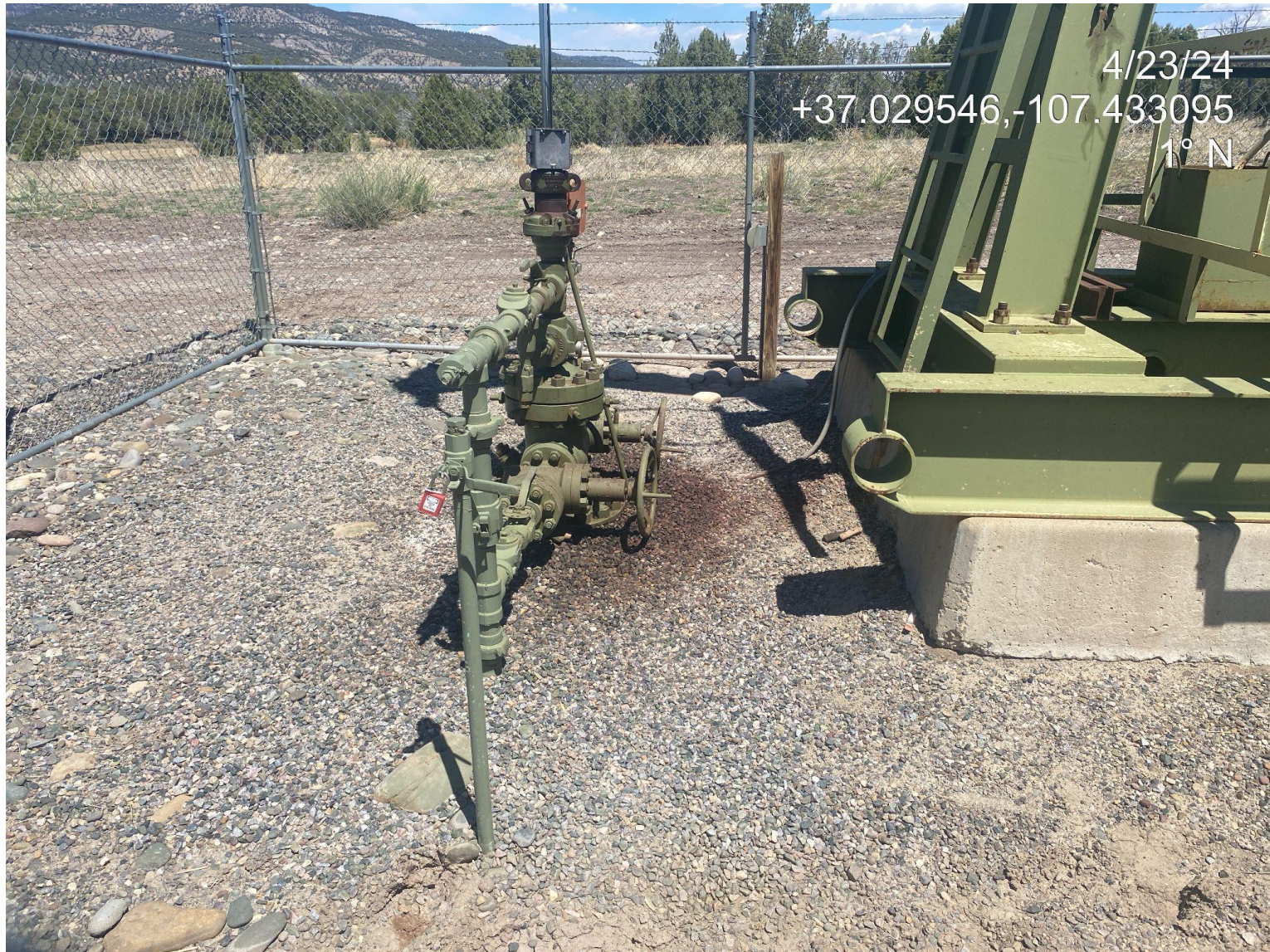
Photo 5. Impacted surface material observed at the well head.
