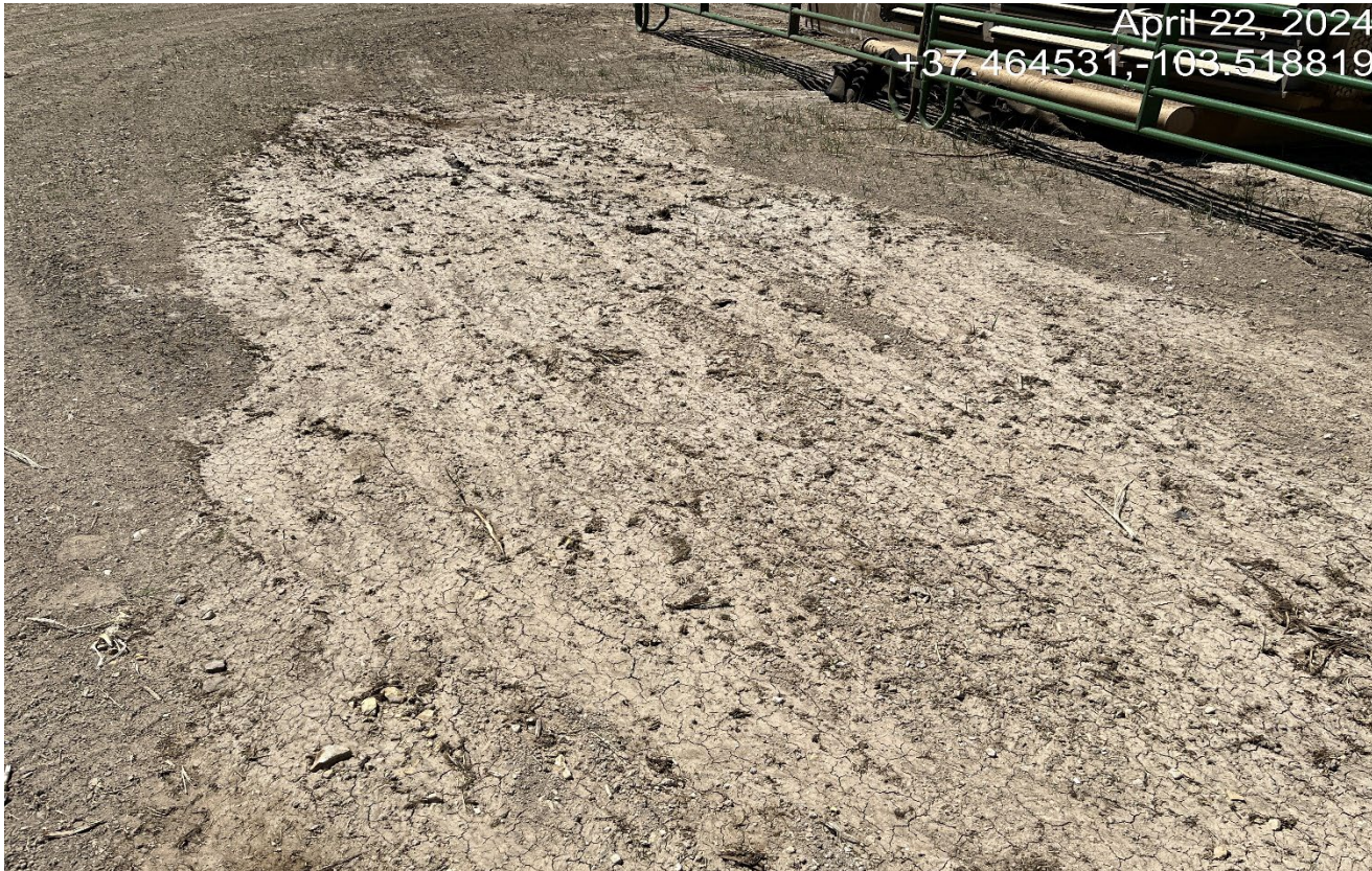
Photo 10. View of stained soil at the back side of the compressor about 6'x5'.
