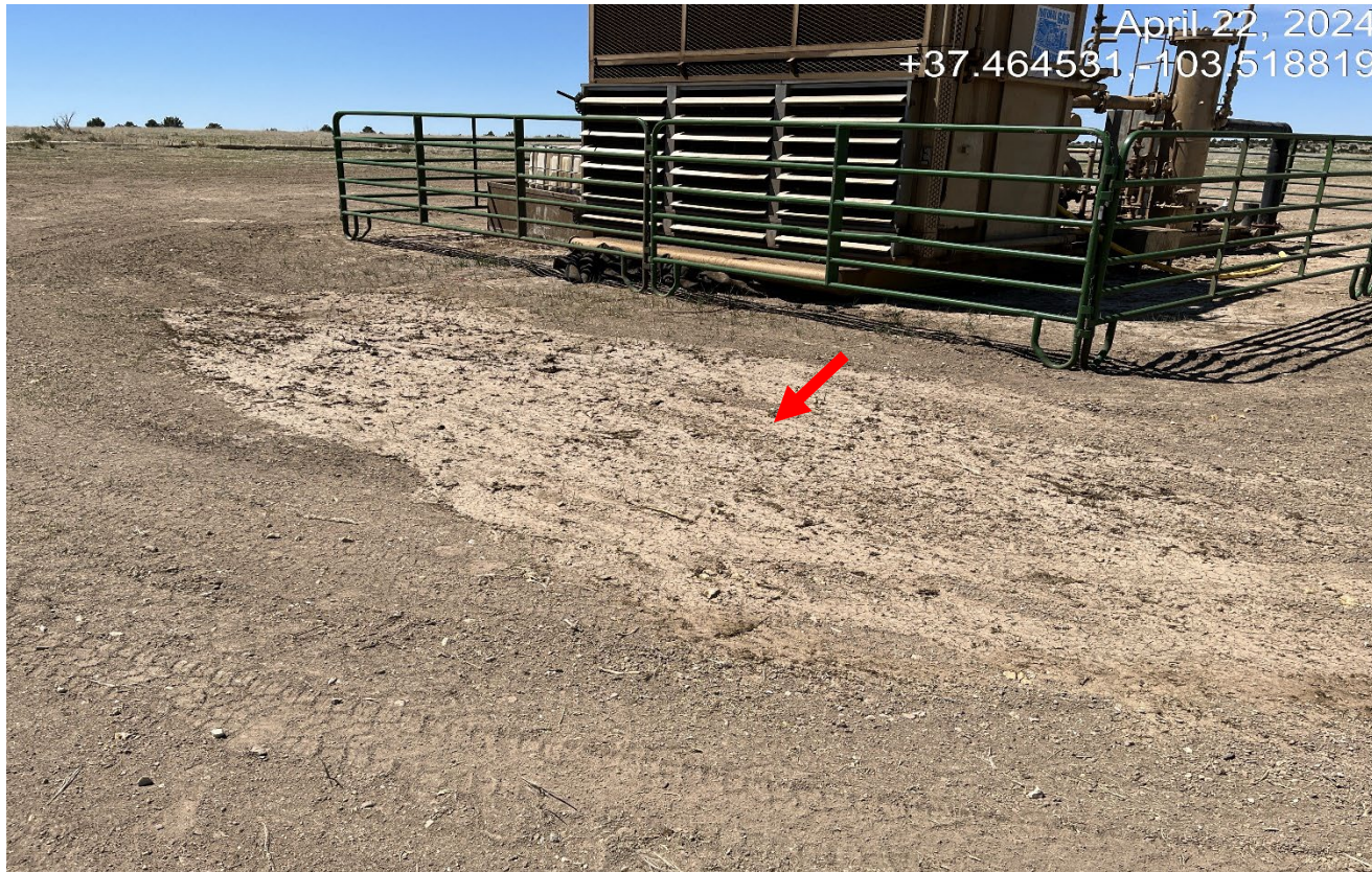
Photo 9. It appears there was a leak at the backside of the engine compressor.
