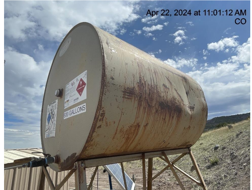
Photo # 4576 Methanol tank improperly labeled/lacks required information
