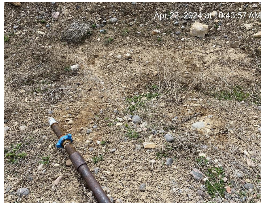
Open end load line. Staining in unauthorized pit.
