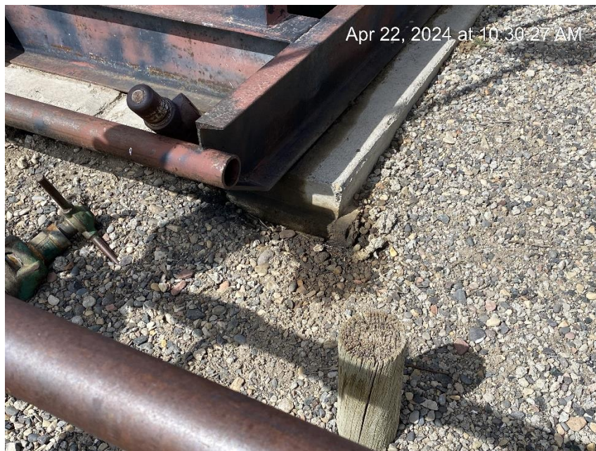
Stained soil from leaking equipment
