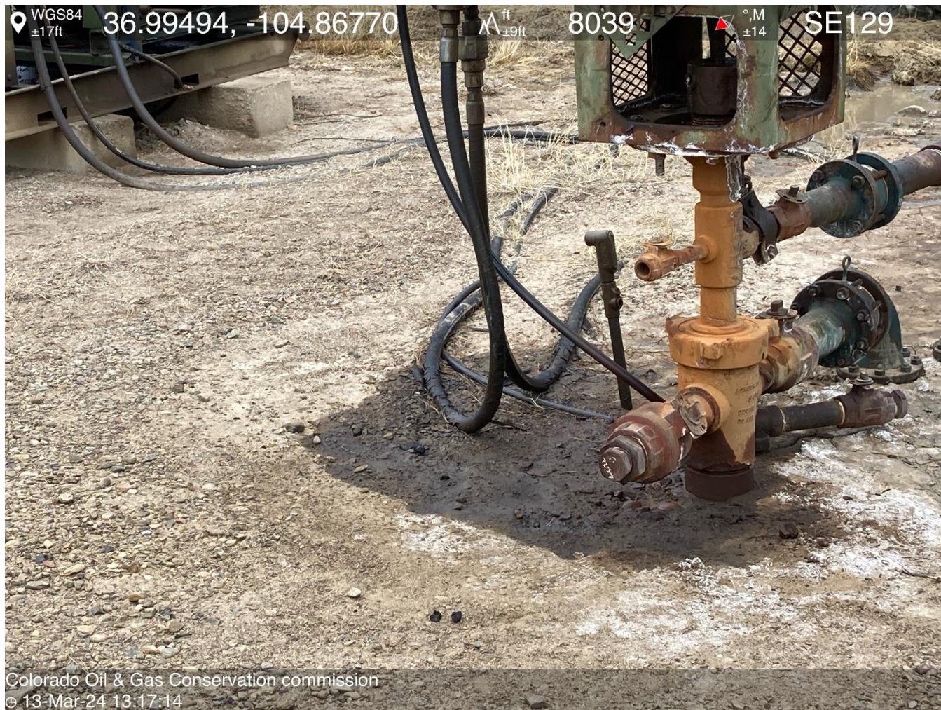
PHOTO 4: AREA OF IMPACTED SOIL UNDER DRIVE HEAD. Conduct maintenance on equipment, cleanup stained material and review self inspection processes. COMPLY WITH RULE 1002,.(2).D. CA DATE 5-22-2024.
