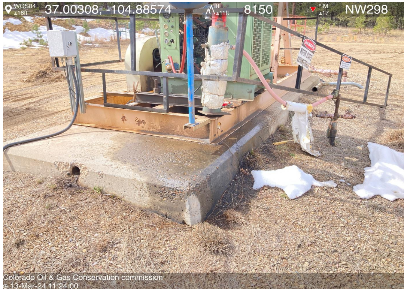
PHOTO 4: LEAKS ON PUMP JACK PRIME MOVER HAS RESULTED IN IMPACTED SOIL JUST OFF PUMP JACK PAD. Conduct maintenance on equipment, cleanup stained material and review self inspection processes. COMPLY WITH RULE 1002.(2).D AND Securely fasten all valves, pipes, fittings, and Production Facilities to ensure good mechanical condition, inspect at regular intervals and maintain in good mechanical condition per Rule 608.e. (i>e REPAIR LEAKS) CA DATE 5-22-2024.
