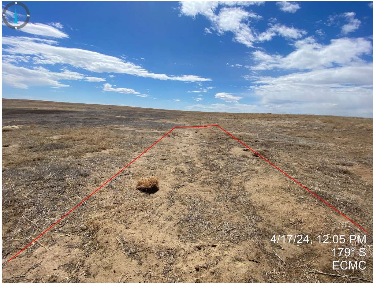
Photo 1. Access road does not appear to be properly stabilized as the road is primarily bare/exposed soil.
