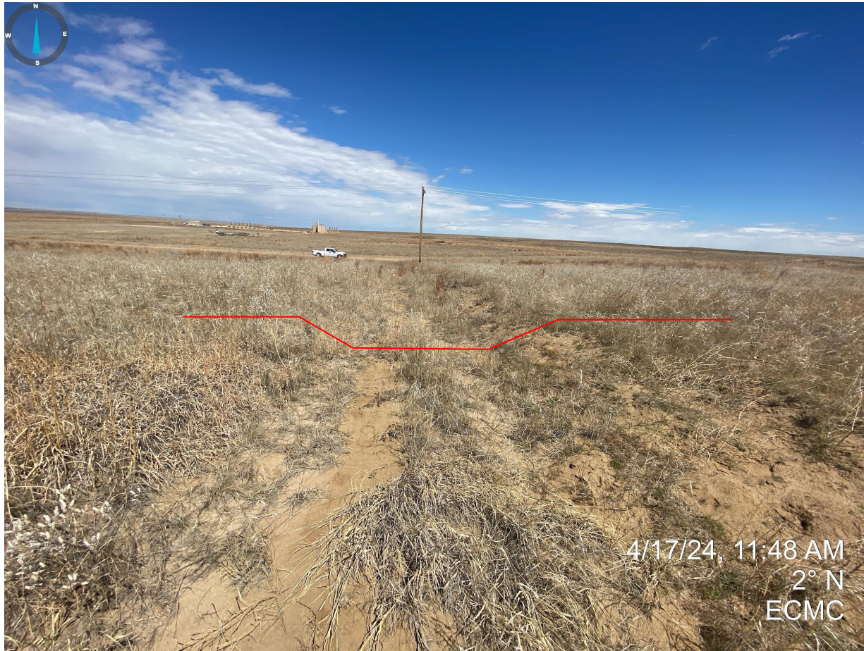
Photo 2. Access road has not been recontoured/graded to reflect adjacent topography.
