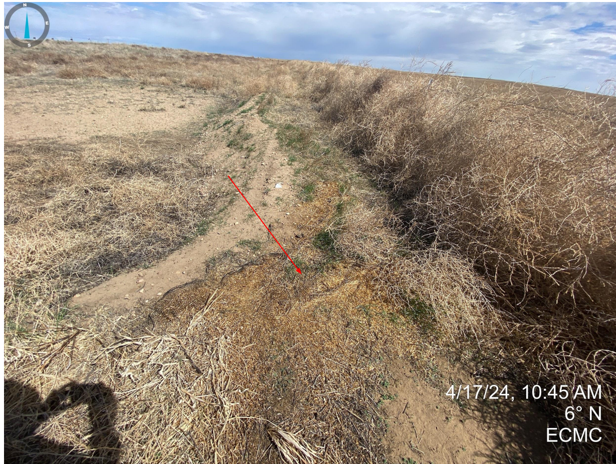
Photo 3. Degraded straw wattle at the SE corner of the location (sediment trap) is now considered debris.
