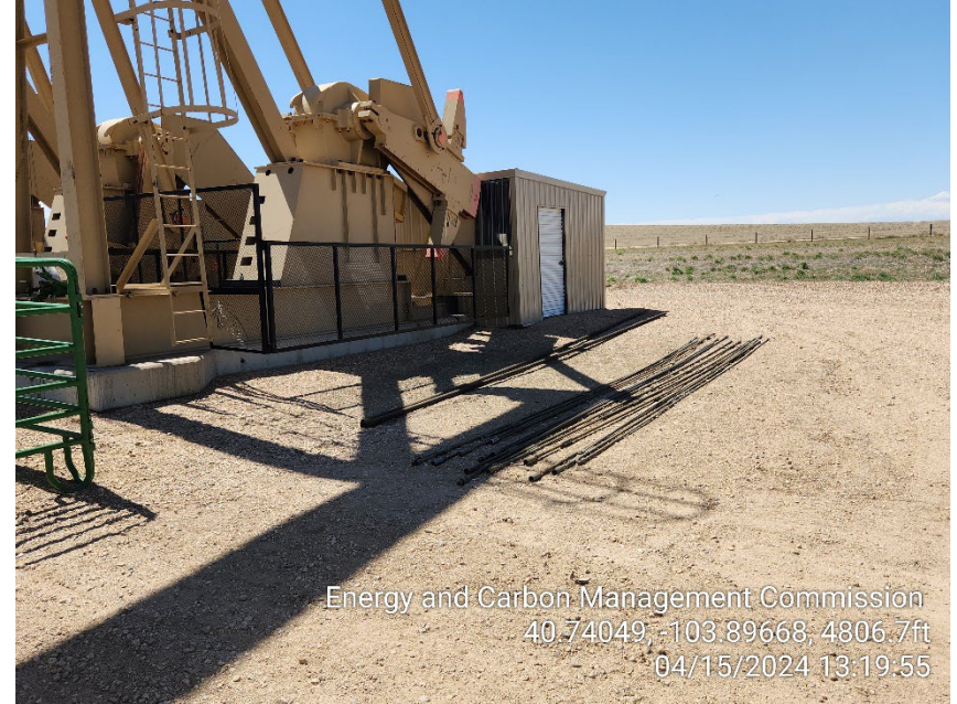
Photo 8 – Unused Rods and Tubing
