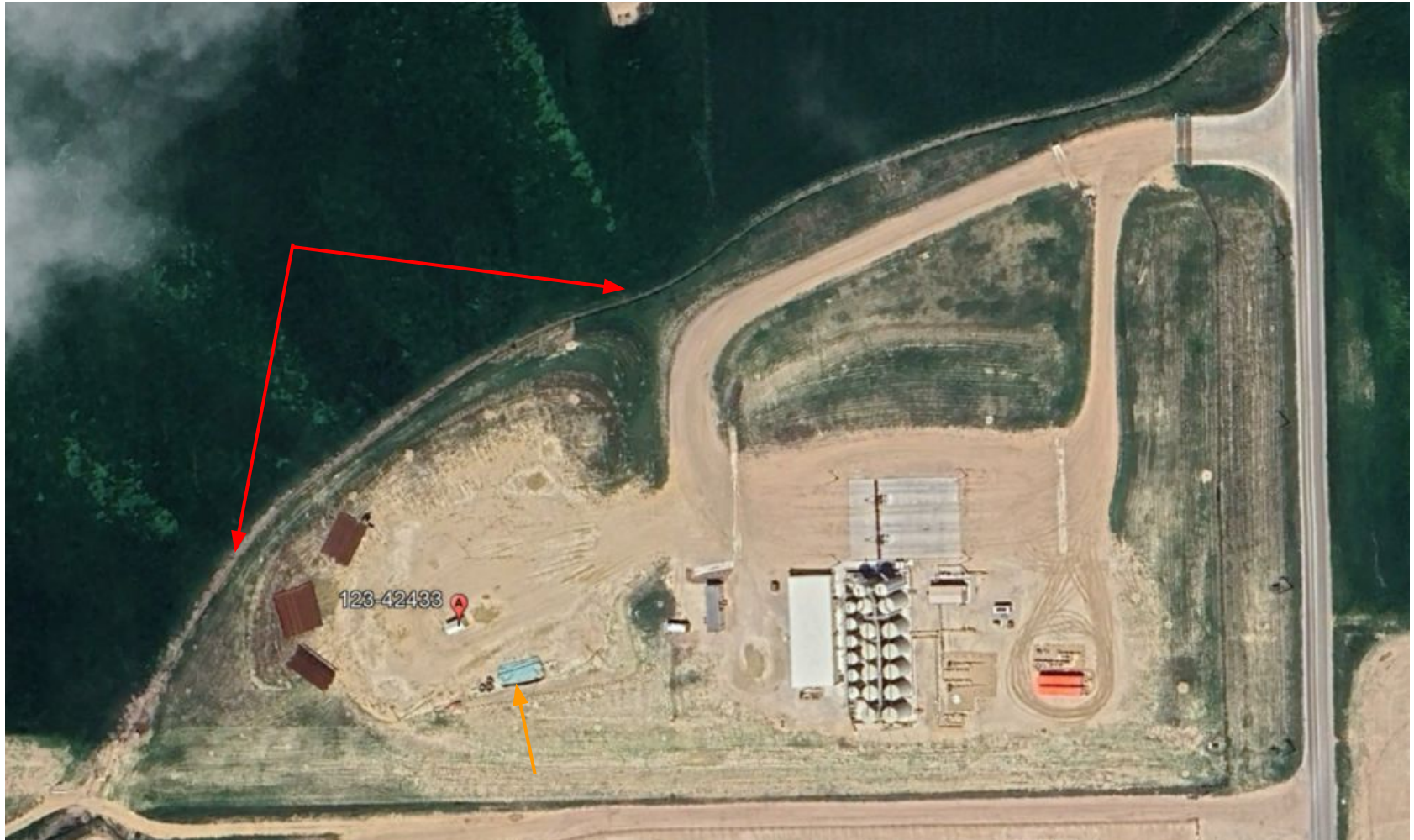
Photo 1. Google Earth aerial imagery from 5/24/2023 illustrating the location. Operator has failed to install perimeter stormwater BMPs while conducting interim reclamation activities.
