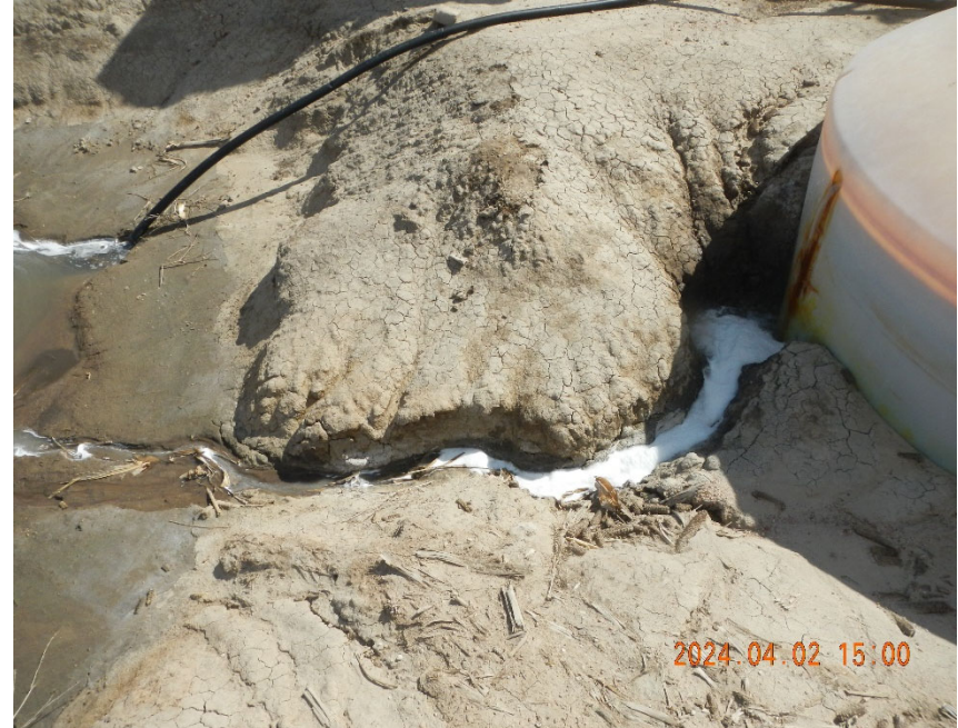
10. Erosion channel from tank to pit.
