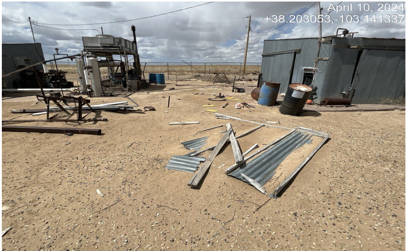
Photo 5. Facing west at the sheds and various equipment which are in disrepair. There is chemical barrels with no containment and various debris laying on the ground.
