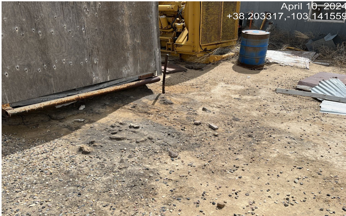
Photo 12. There are stained soils near this shed and engine compressor. There is chemical barrels with no containment and various debris laying on the ground.
