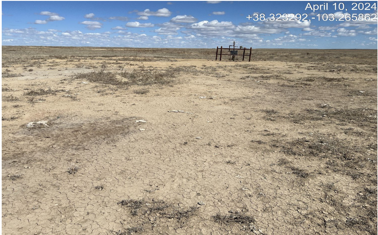
Photo 1. Facing north toward the wellsite. The area around the well has not revegetated. There is bare soils extending approximately 100 ft. out from the well that needs to be reclaimed.
