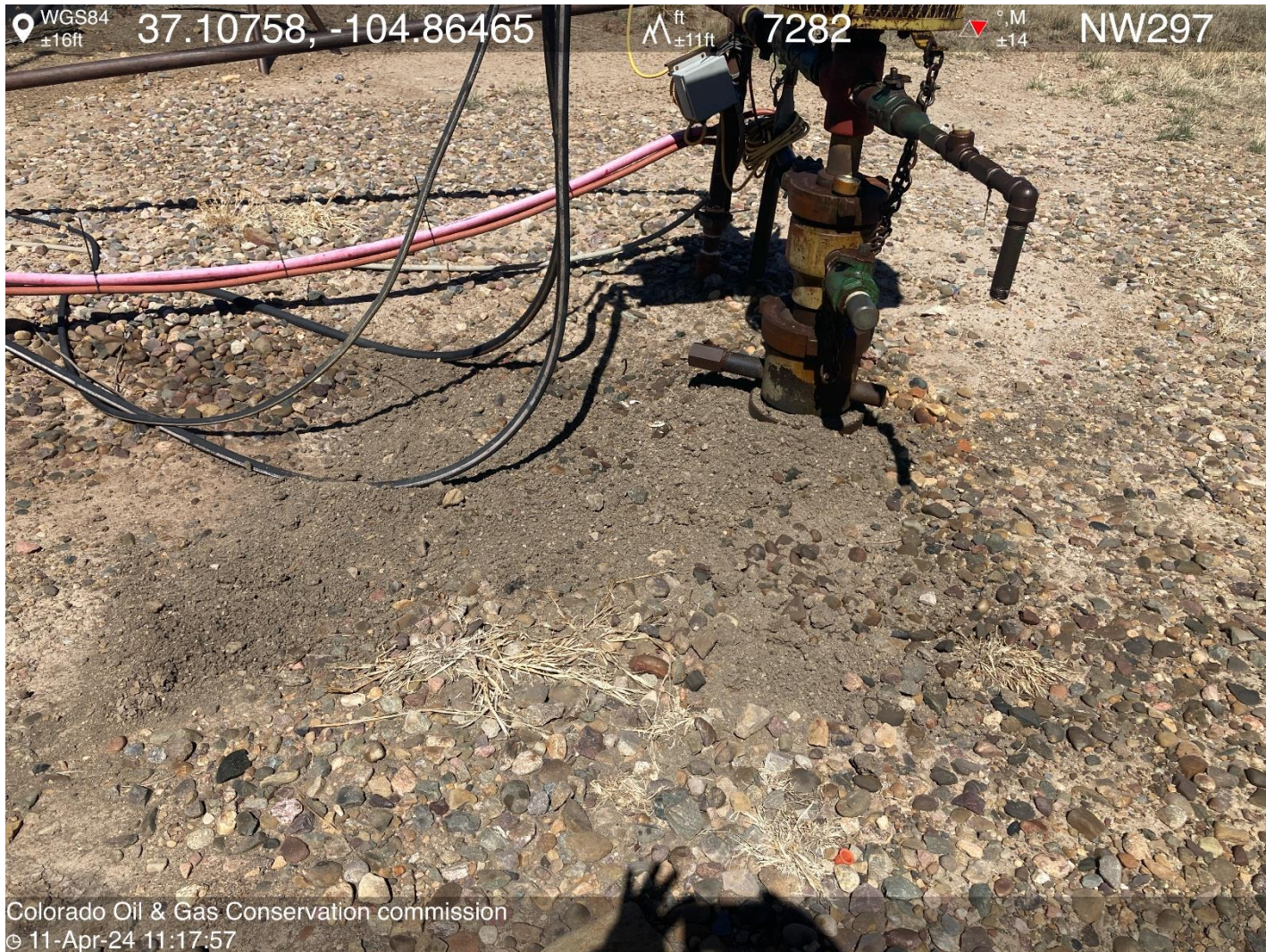
PHOTO 5: AREA OF IMPACTED SOIL NEAR WELLHEAD APPEARS TO BE HYDRAULIC OIL FROM LEAKING DRIVEHEAD (IT APPEARS THAT OPERATOR ATTEMPTED TO COVER IMPACTED SOIL WITH SOIL FROM PIT BERM). Conduct maintenance on equipment, cleanup stained material and review self inspection processes. COMPLY WITH RULE 1002, (2).D. CA DATE 4-18-2024.
