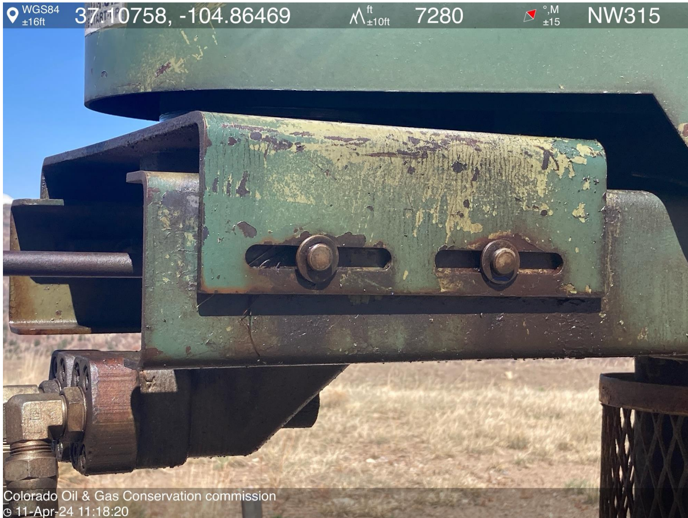
PHOTO 4: APPEARS TO BE A HYDRAULIC LEAK ON THE DRIVE HEAD. Securely fasten all valves, pipes, fittings, and Production Facilities to ensure good mechanical condition, inspect at regular intervals and maintain in good mechanical condition per Rule 608.e. CA DATE 4-18-2024.
