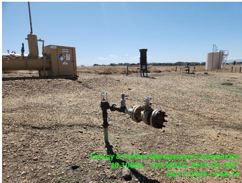
Photo 13 Flow line needs to be retagged.
