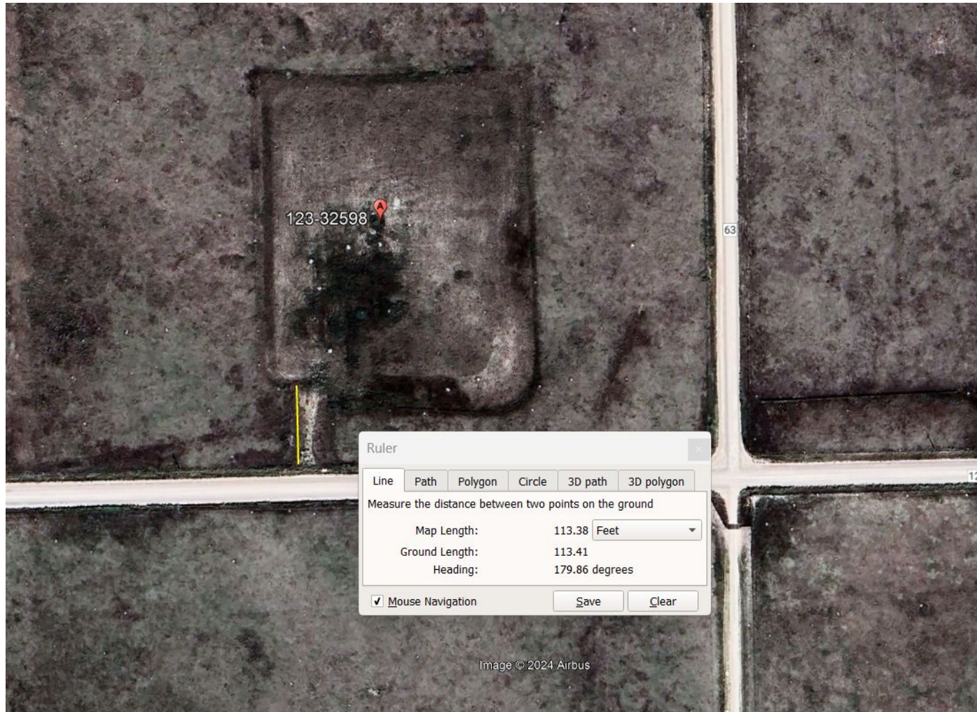
Photo 1. Google Earth aerial imagery from 9/3/2023 illustrating the location. Operator has performed final reclamation activities; however, Operator has left an approximate 100' section of access road in-place.
