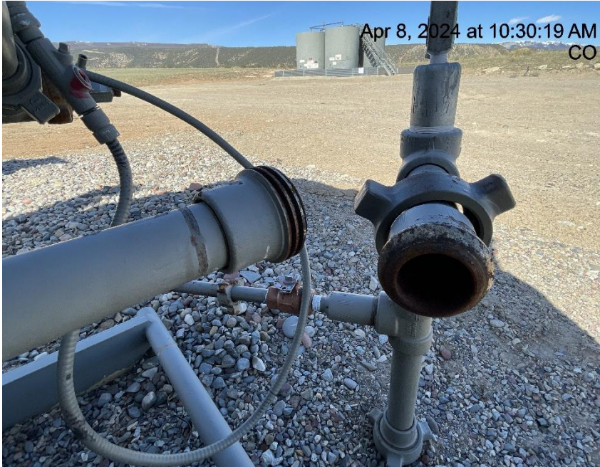
Photo # 2995 Open ended pipping on separator unit/wildlife hazard/available for entry by wildlife
