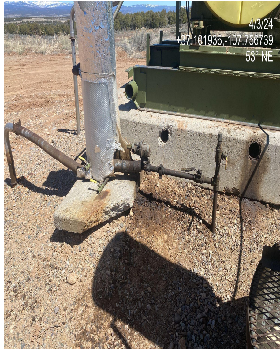
Photo 3. View of stained material at both pump jack mufflers.
