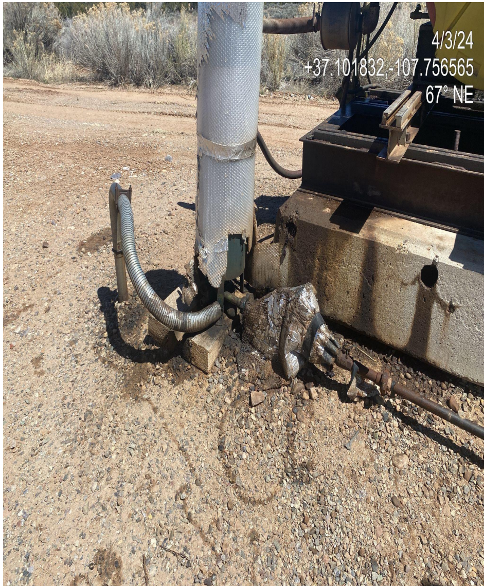
Photo 3. View of stained material at both pump jack mufflers.
