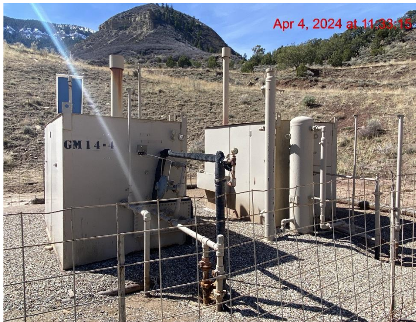
Separator/Dehydrator – Photo #00402
