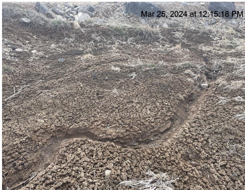
Photo # 1273 Ditch/BMP near entrance to location needs maintenance/small breach in ditch allowing sediment transport from ditch into the interim area & causing more erosion & sediment transport in the interim area itself.
