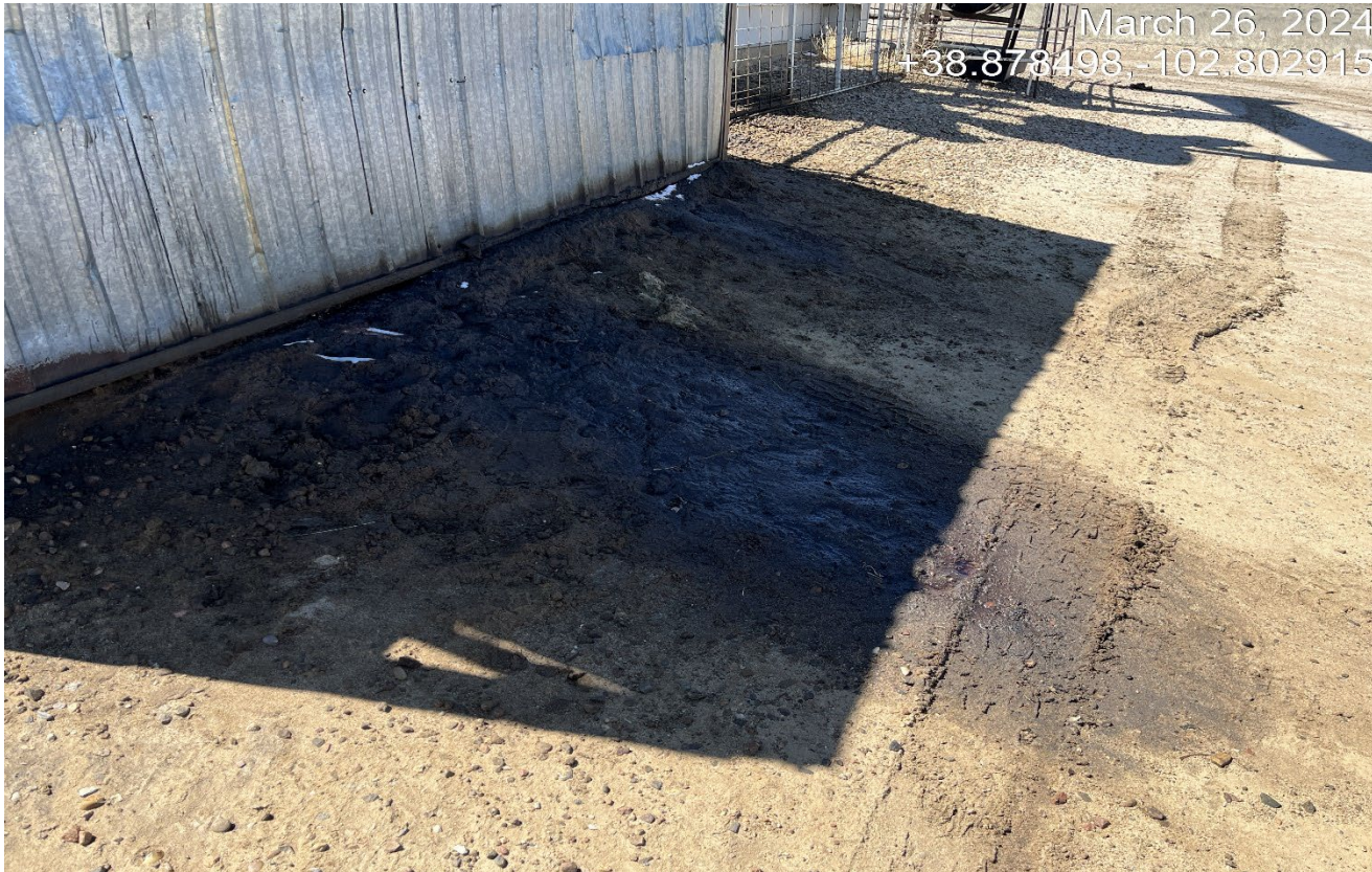
Photo 6. There is lube oil leaking out of the pumpjack engine that must be controlled and cleaned up.
