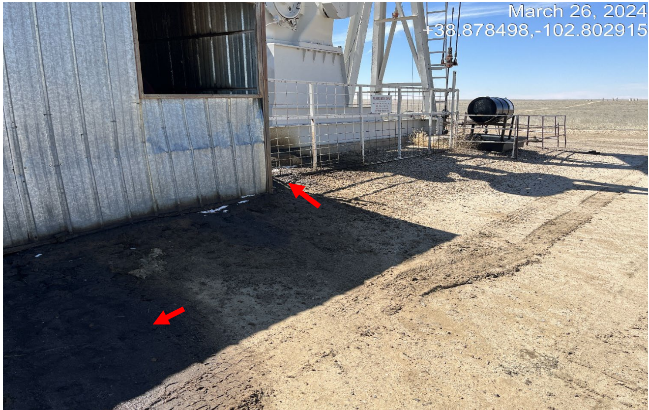
Photo 8. The red arrows point to oily impacted soils coming from the pumpjack.
