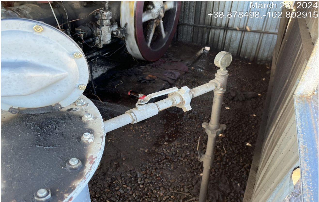
Photo 7. View of inside the shed where oil is leaking out of the pumpjack engine.
