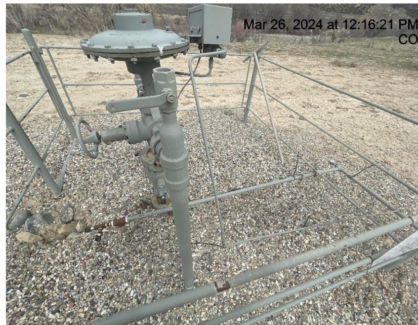
Photo # 1535 KNIGHT W-6-4 bradenhead tied into flowline/No Form 4 Sundry
