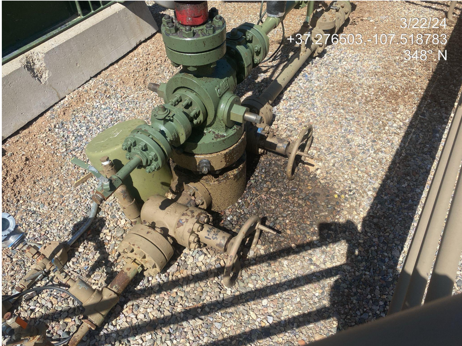
Photo 3. Impacted material observed at the well head.
