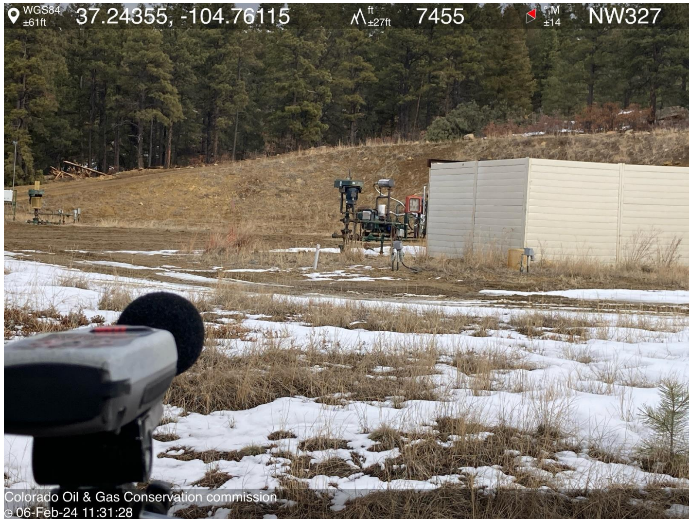
PHOTO 5: METER SET 94.5' FROM COMPRESSOR
