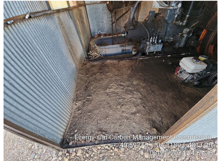
Photo 4 – Gas Engine – Stained Soil
