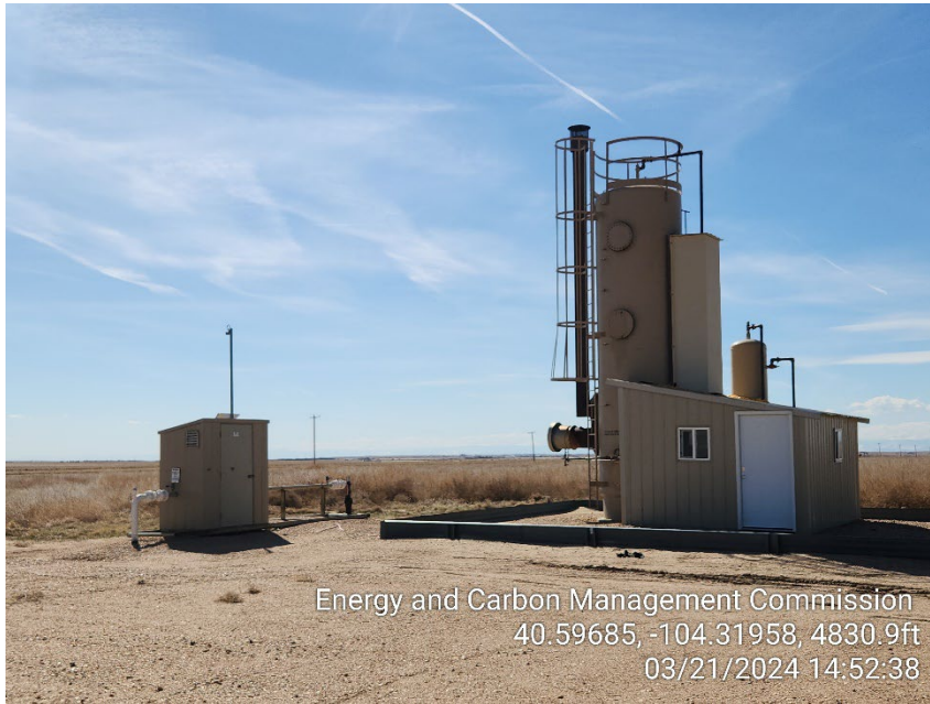
Photo 9 – Heater Treater and Gas Meter
