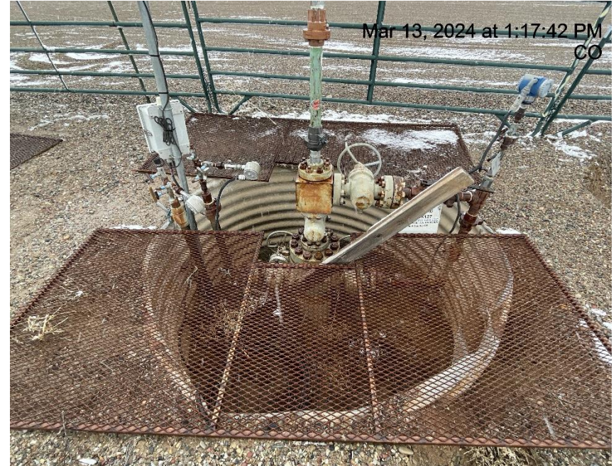
Photo # 9871 Cellar cover not properly installed/wildlife & personnel hazard & wildlife egress not properly installed.
